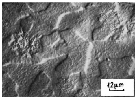
Fig. 6. Electromicroscopic photo of brittle fracture of urethane elastomer obtained in test R-23 (sodium derivative of ethanediol).
